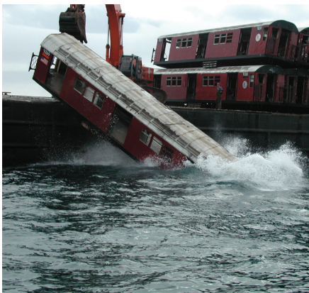
Redbird subway cars donated by the New York City Transit Authority and deployed as artificial reef material at Reef CCA-JY in December of 2002. Courtesy of GA DNR CRD
